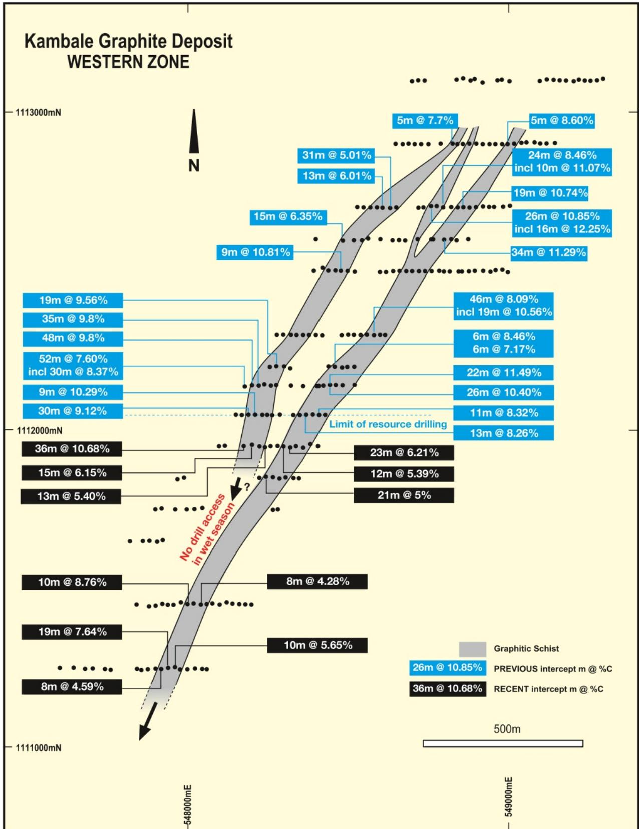
**Figure 3: RC drill cross sections of the Western Zone of Kambale Prospect with significant graphite intercepts**
